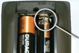
Corrosion you CAN see
