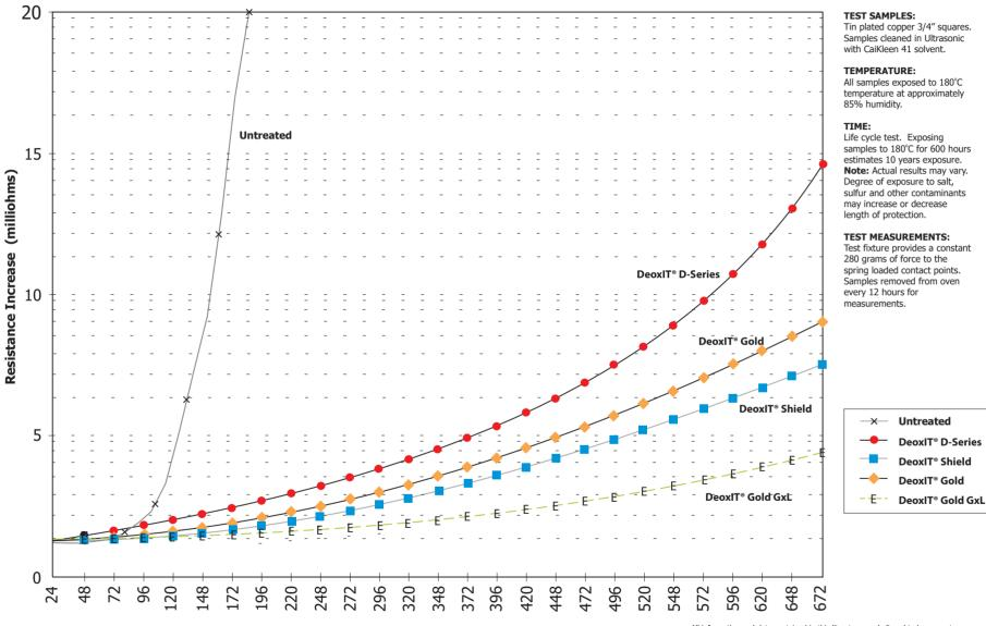
September 2008 Bulletin No.: CH-DPP-11 **Time (hours)** at a constant temperature of 180° C (Simulates 10 year life cycle.)
